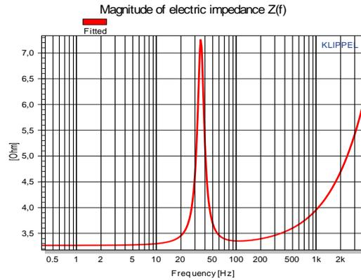
The maximum in the electrical input impedance  $Z(f)$  reveals the fundamental resonance. The fitting of the modeled curve based on the estimated lumped parameters with the measured impedance curve is the most reliable way for estimating the resonance frequency and other small signal parameters.
