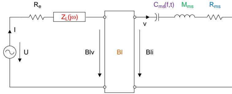
The moving mass  $M_{ms}$  and the compliance  $C_{ms}$  generate a vibrating system with a resonance frequency
